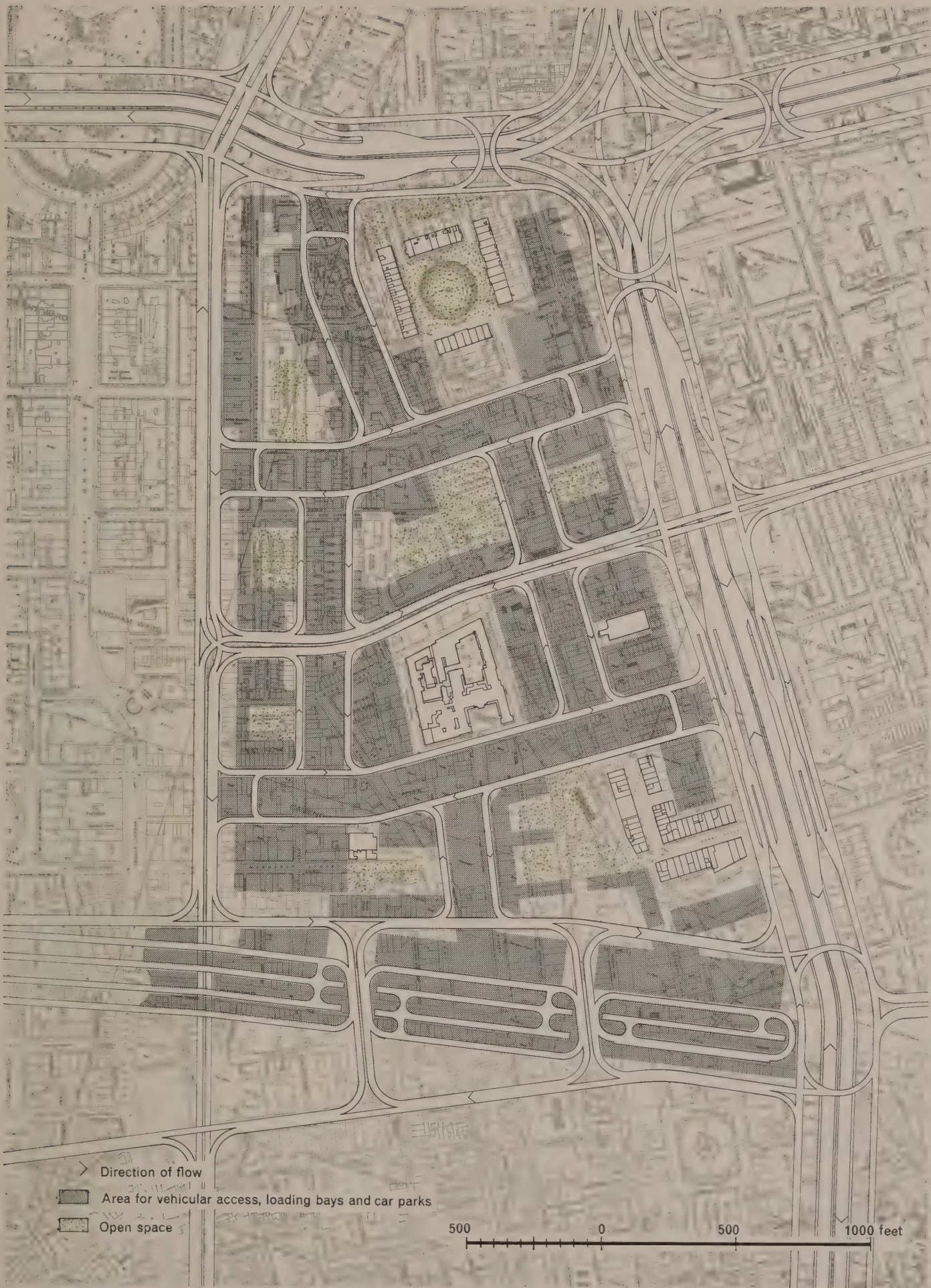
192 The design for partial redevelopment—plan at ground level showing the primary, district and local distribution road system together with the parking and service areas.
